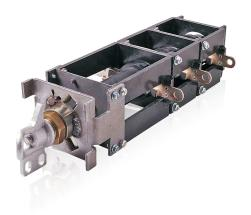
The ABB LBOR-II switch is a manually operated, two position, load make or break, oil immersed, rotary switch. It is designed for use with distribution transformers (pad-mounted or submersible) and self contained distribution switchgear.
