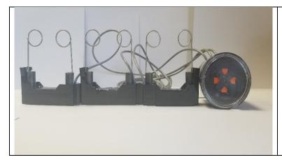
The EC-31 is a three phase, cable mounted unit with remote indicator, designed for use on insulated cable. Bails and tie wraps are included for simple installation. Unit will only reset when the current in each of the three sensors exceeds the reset current. An optional mounting kit with viewing window provides easy field installation in a transformer housing.
