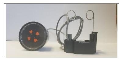
The EC-11 faulted circuit indicator is a single phase, cable mounted unit with remote indicator, designed for use on the cable as well as the elbow. It is manually applied, and is used for underground applications in pad mount transformers. An optional mounting kit with viewing window provides easy field installation in a transformer housing.
