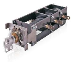
The Hitachi ABB Power Grids Distribution Transformer Components LBOR-II switch is a manually operated, two position, load make or break, oil immersed, rotary switch. It is designed for use with distribution transformers (pad-mounted or submersible) and self contained distribution switchgear.
